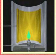
Sample components enter at the base of the detector. They mix with hydrogen and enter the flame.
